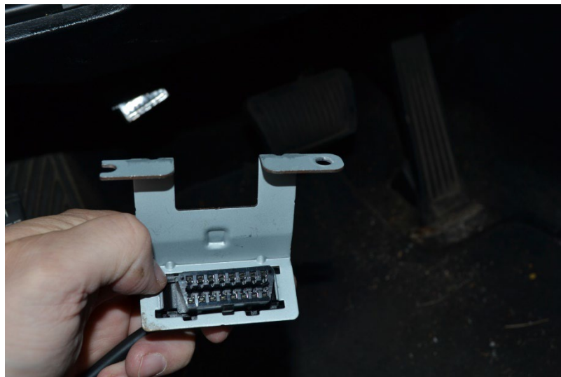
Figure 6 - OBD replicator port inserted in bracket
