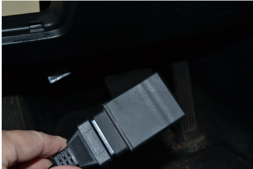
Figure 5 – Connecting GPS tracker to Y-Cable
