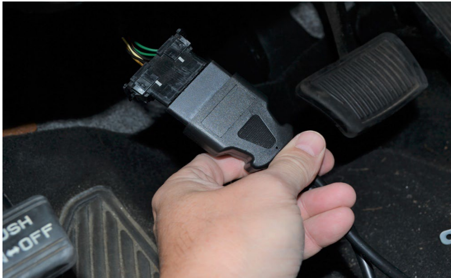
Figure 5 – Connecting Y-Cable to vehicle OBD port
